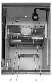
**8** Undo and remove the socket cap screws (E) on the rear knife support rule (F).
